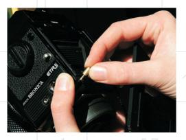
The image to the left shows how to fit the Silvestri adapter cod. 7010. Use the provided pin to unlock the volè's feeler pin in the following way: holding pressed the unlocking button of the film holder, push with the pin the feeler pin and hold it pushed.
